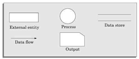
Figure 6.2: Symbols used for designing DFDs.
