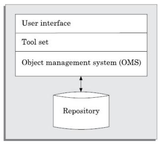
Figure 12.2: Architecture of a modern CASE environment.
