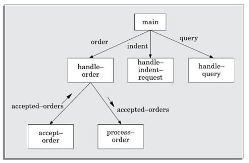
Figure 6.22: Structure chart for Example 6.9.
