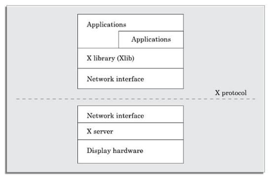
Figure 9.6: Architecture of the X System.
