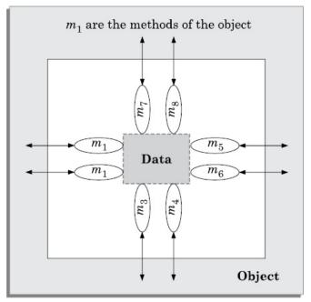
Figure 7.2: A model of an object
