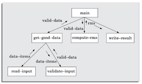
Figure 6.19: Structure chart for Example 6.6.
