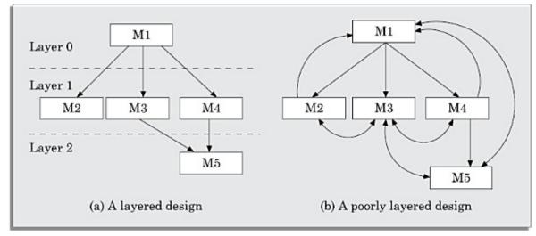
Figure 6.18: Examples of properly and poorly layered designs.
