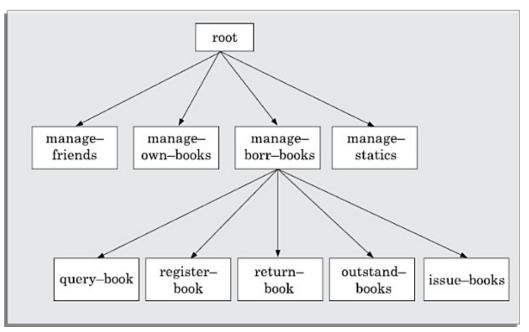
Figure 6.23: Structure chart for Example 6.10.
