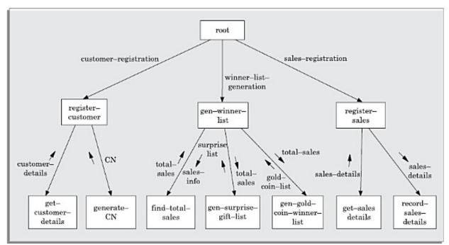
Figure 6.21: Structure chart for Example 6.8.
