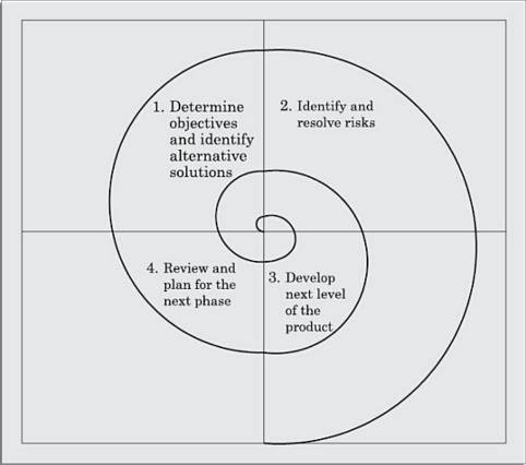
Figure 2.10: Spiral model of software development.
