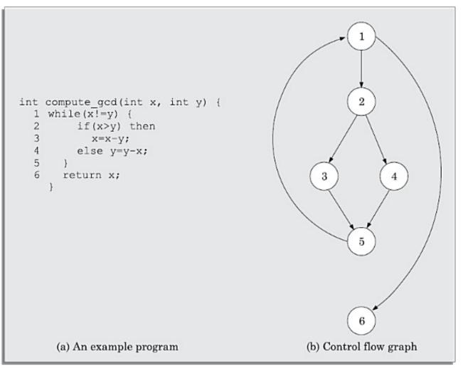
Figure 10.7: Control flow diagram of an example program.
