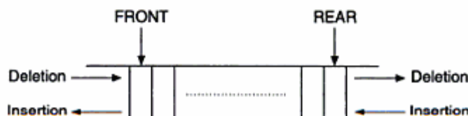
Figure 5.9 A deque structure.
